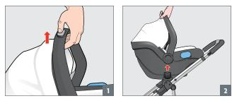
**STEP 1:** Engage and hold the stroller release button on the top of the carry handle.
