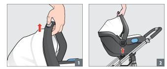
**STEP 1:** Engage and hold the stroller release button on the top of the carry handle.
